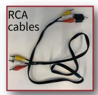
1.Connect the Elgato device to the red, yellow, and white RCA cables. Make sure the colours match.
